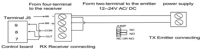
**Fig.9 infrared Schematic diagram**
